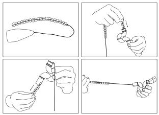
How to clean the inner tubes (headjoint, bodyjoint, and footjoint)
